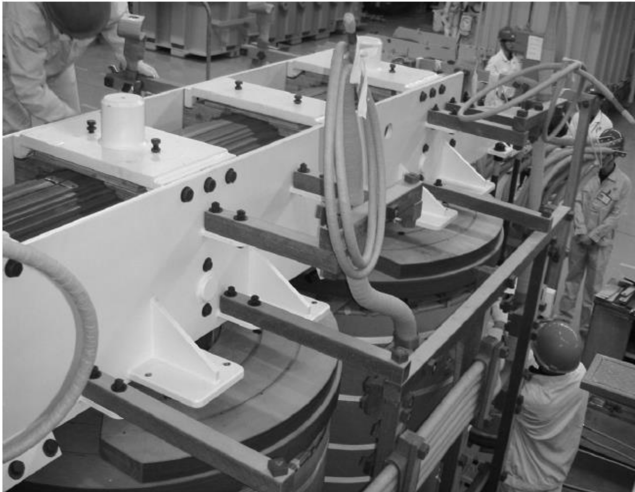
FIGURE 1.16 (See color insert following page 338.) Top view of a clamping structure for a three-phase transformer.
